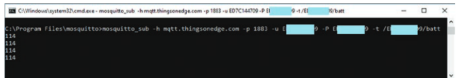
Screen5: this command, issued after installing the 'mosquitto' software, allows the IOT Cricket's messages to be checked and monitored. The 'batt' topic name can be replaced with any of the others that are supported, or the '#' MQTT wildcard to see all messages.
